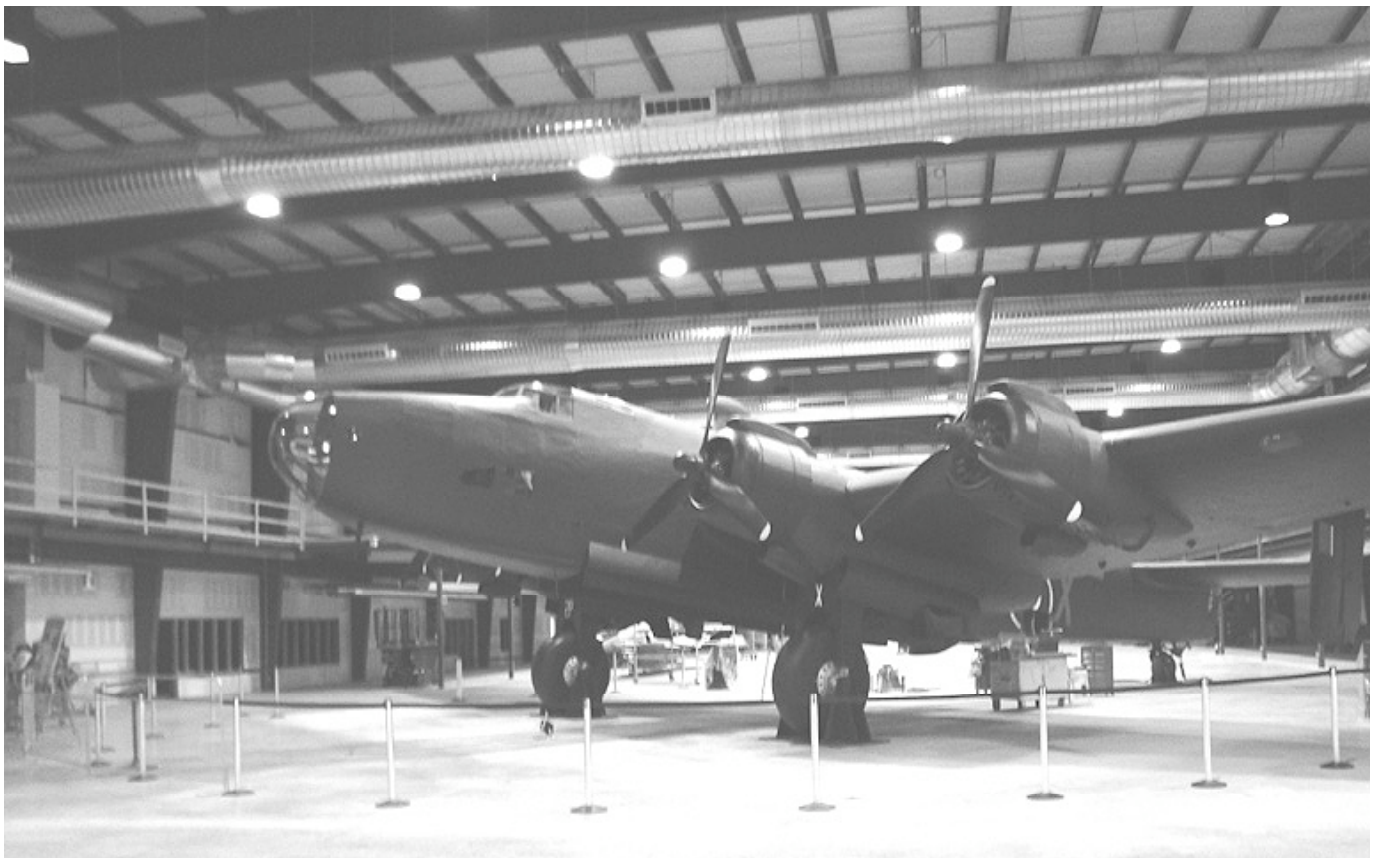
View of Halifax NA337 sporting new nose-glass and 12 new propeller blades.
